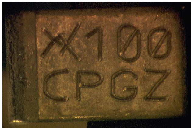
Figure 9. This part is laser marked, but the font is hand-written.
